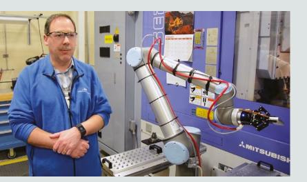
We've added capacity by being able to run the machine during unattended hours, but it also freed up skilled workers to do highervalue tasks as opposed to loading and unloading the machine.
